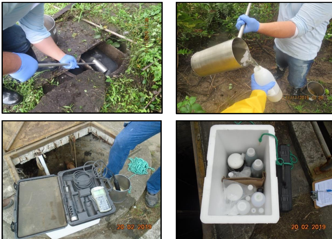
Figure 38. Effluents samples collection in order to evaluate physical-chemical and biological parameters.
