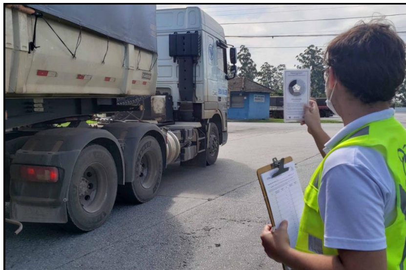
Figure 37. Blacksmoke monitoring with the methodology known as “Ringelmann scale”.
