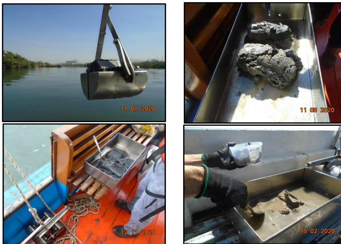
Figure 21. Sampling and storage of sediment collected during a campaign of the Sediment Quality Monitoring Program.
